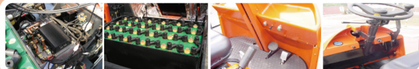
Infinite speed control in forward and reverse | High capacity traction battery | Flexible function and smooth acceleration/deceleration | Human-based design and operator perception system
